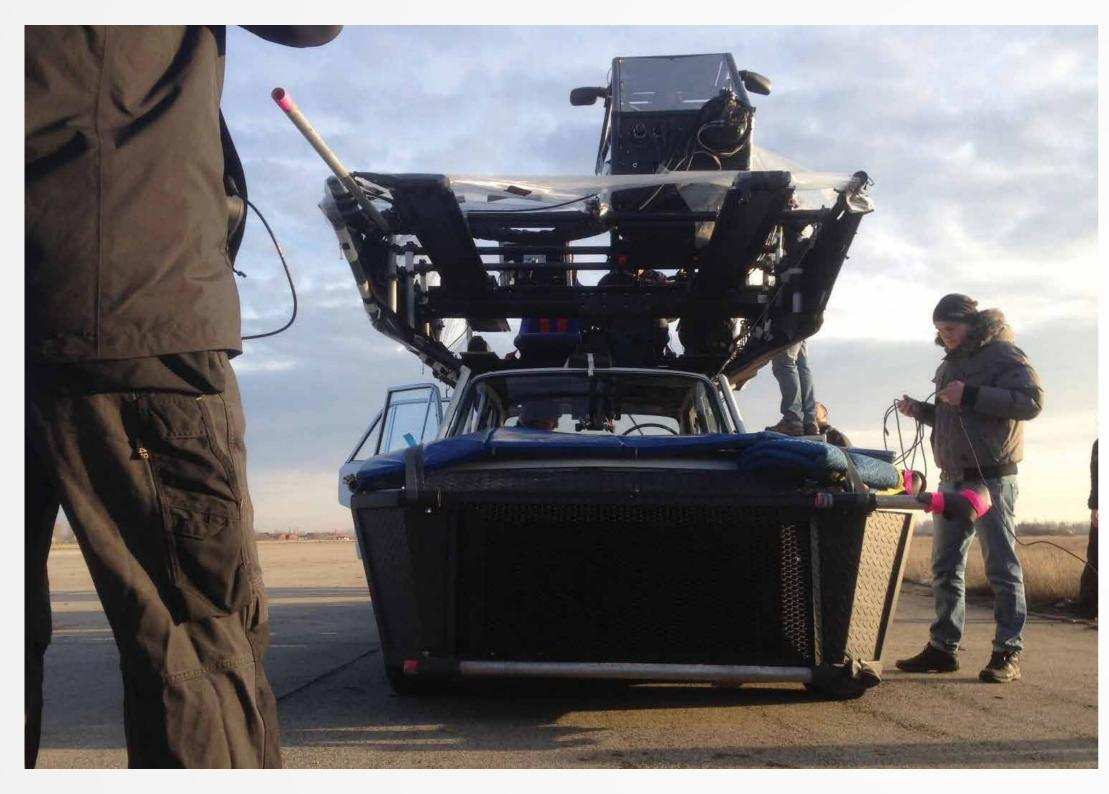
The Grand Track is a fully self-drivable trailer custom developed for the movie industry. With it's V8 350 HP engine and one automatic gear shift system, the Grandtrack is constructed for consistent smooth and steady movements. All the three axes have their own air suspension and shock absorbers with adjustable stiffness.
